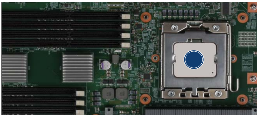
Figure 120: Applying the thermal paste
